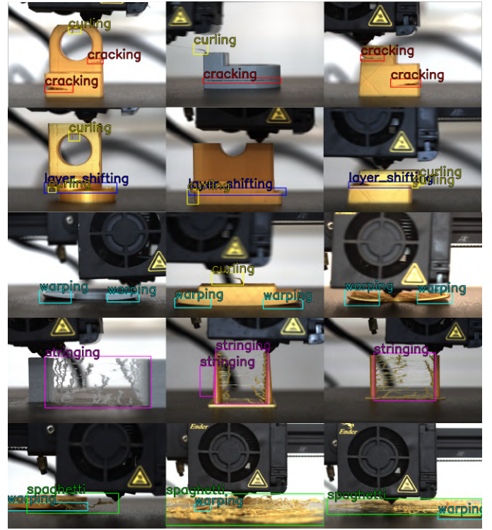
Fig. 2. Final annotated images illustrating various defect types. From top to bottom, the primary class (as the original dataset) for each row is: cracking, layer shifting, warping, stringing, and spaghetti (off-platform).
